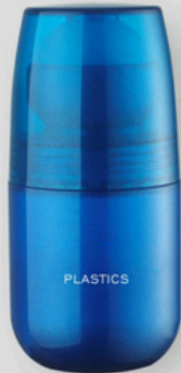
P3003 Volume:50ml Ball Diameter:35.56mm Height:104.6mm Material Cap:PET Bottle:PET Ball:PP
